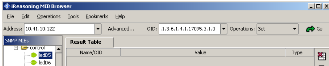
Figure 12: Configuration of a Set Operation
