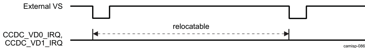
Figure 12-43. CCDC_VD0_IRQ/CCDC_VD1_IRQ Interrupt Behavior When VDPOL = 1
