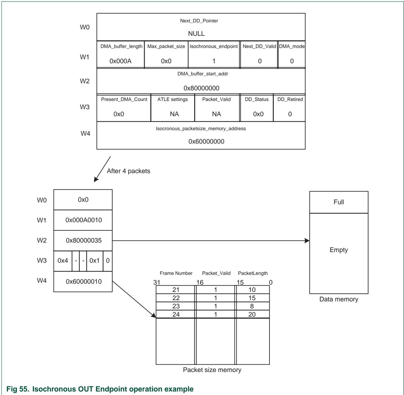
Fig 55. Isochronous OUT Endpoint operation example
