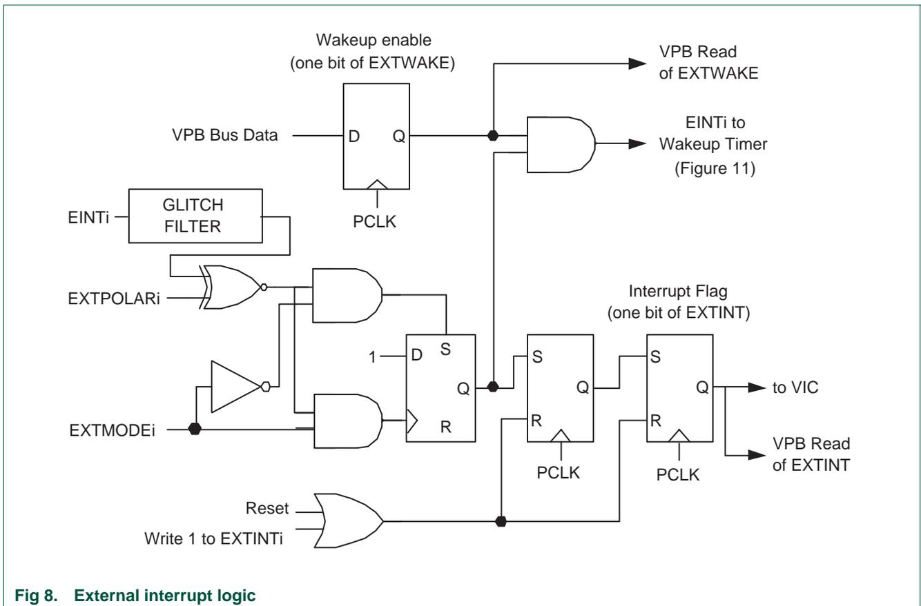
Fig 8. External interrupt logic
