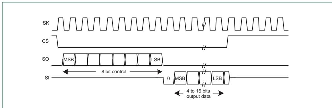
**Fig 47. Microwire frame format (single transfer)**
