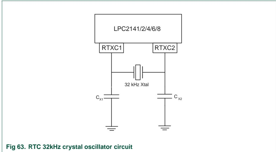
Fig 63. RTC 32kHz crystal oscillator circuit
