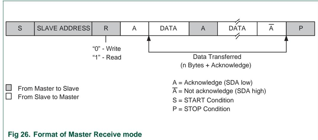
After a repeated START condition, I<sup>2</sup>C may switch to the master transmitter mode.
