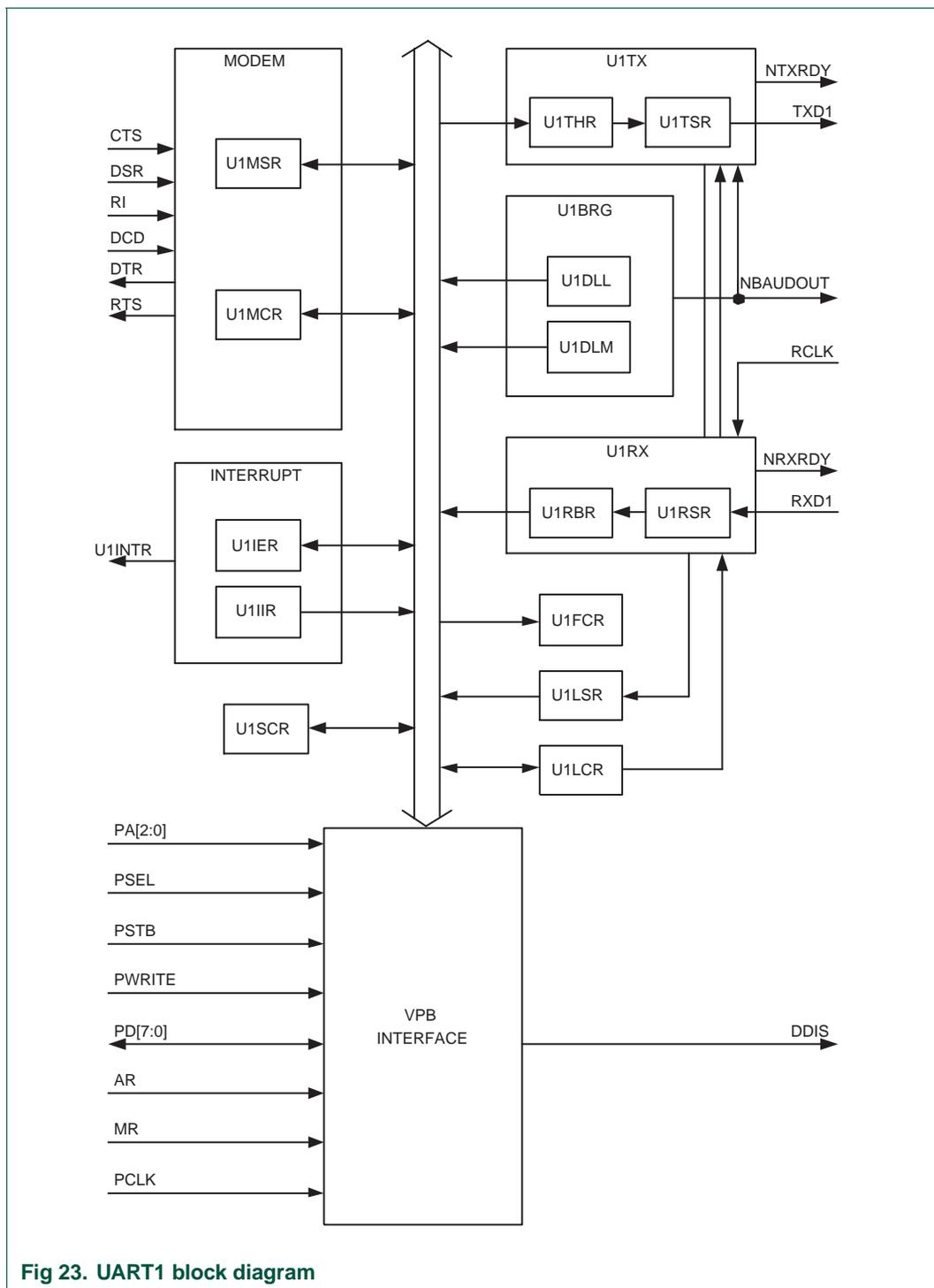
Fig 23. UART1 block diagram
