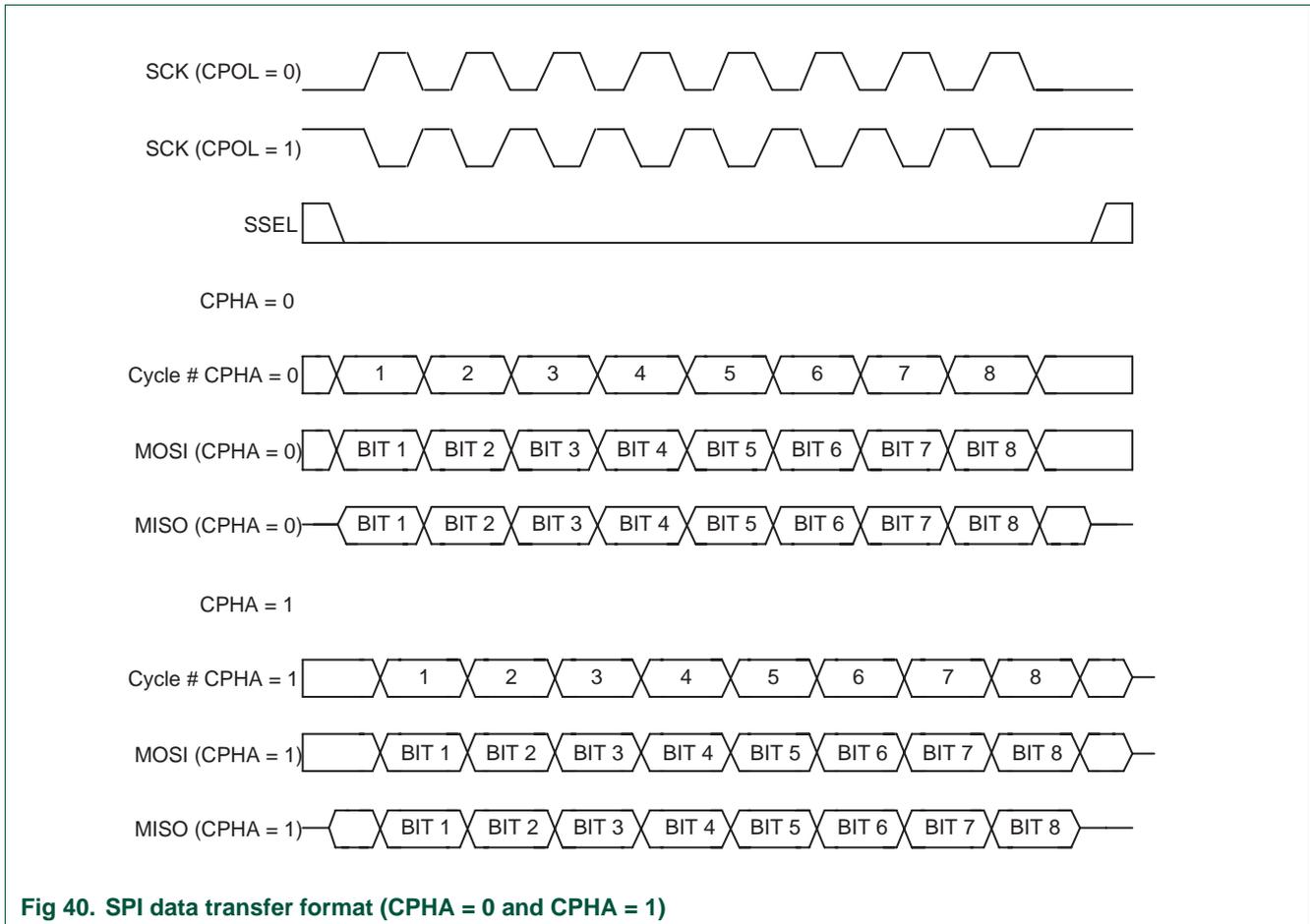
Fig 40. SPI data transfer format (CPHA = 0 and CPHA = 1)
