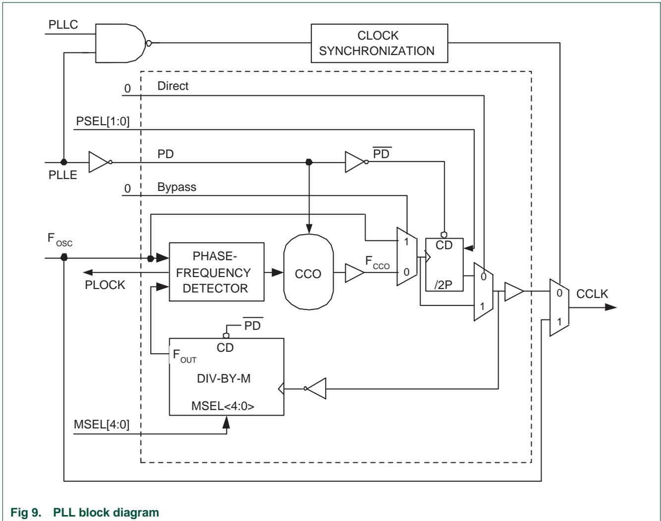
Fig 9. PLL block diagram
