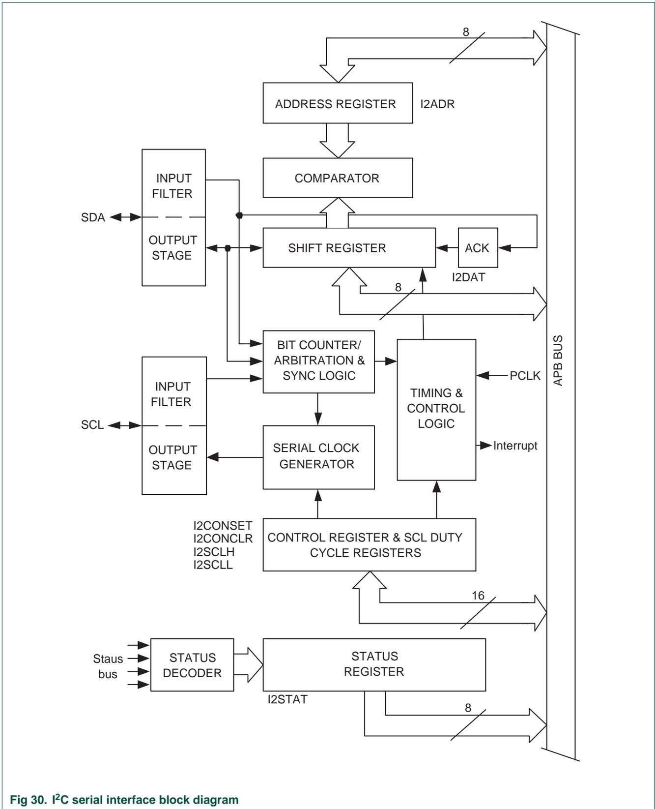
Fig 30. I<sup>2</sup>C serial interface block diagram
