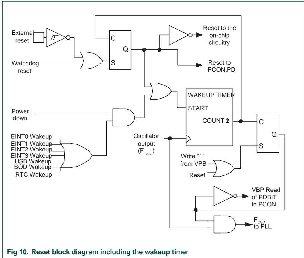
Fig 10. Reset block diagram including the wakeup timer
