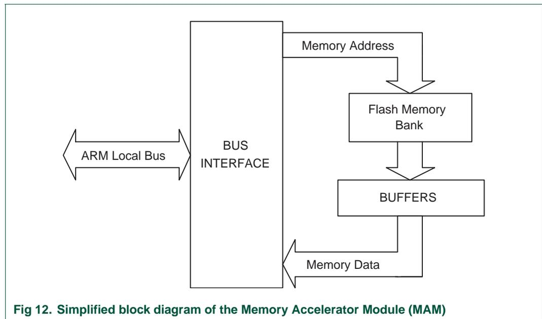
Fig 12. Simplified block diagram of the Memory Accelerator Module (MAM)
