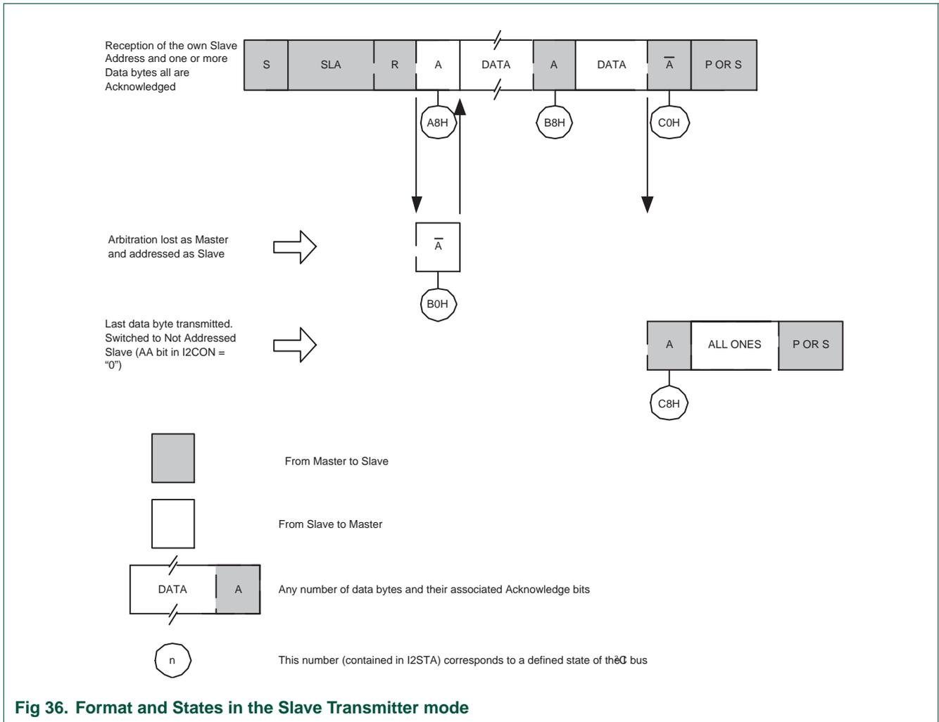
Fig 36. Format and States in the Slave Transmitter mode
