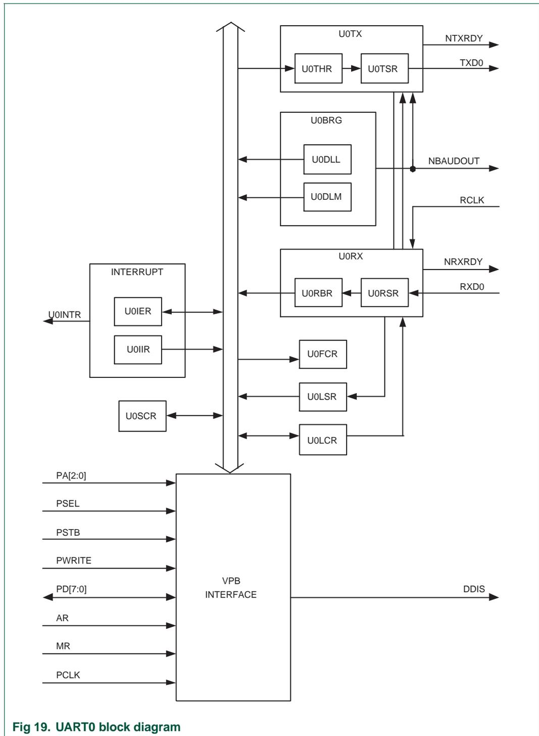
Fig 19. UART0 block diagram
