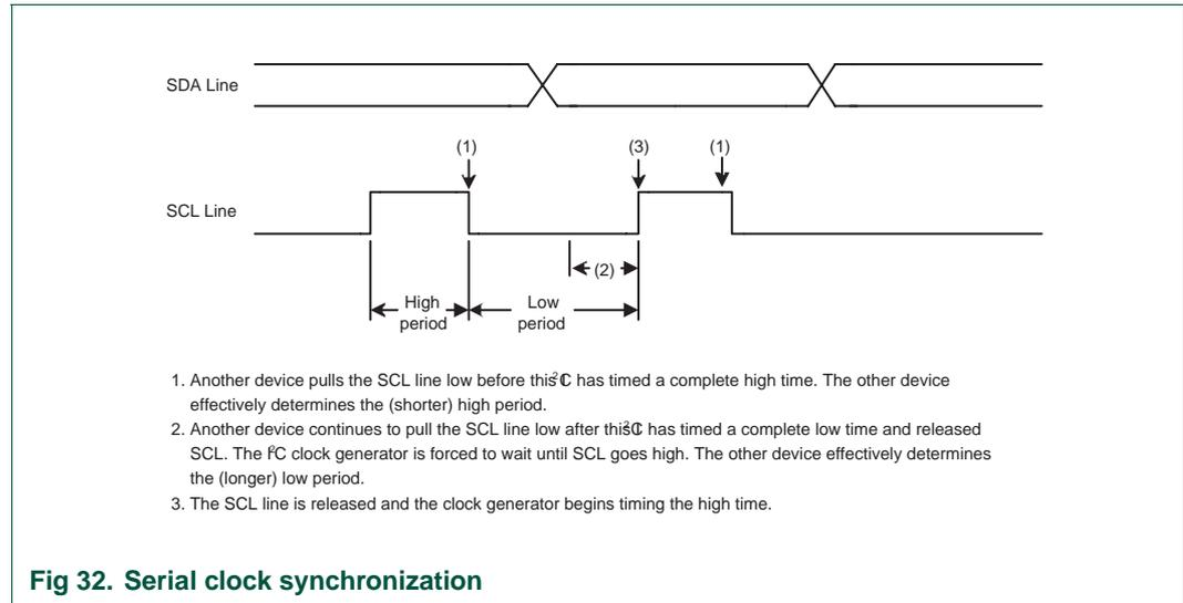
**Fig 32. Serial clock synchronization**
