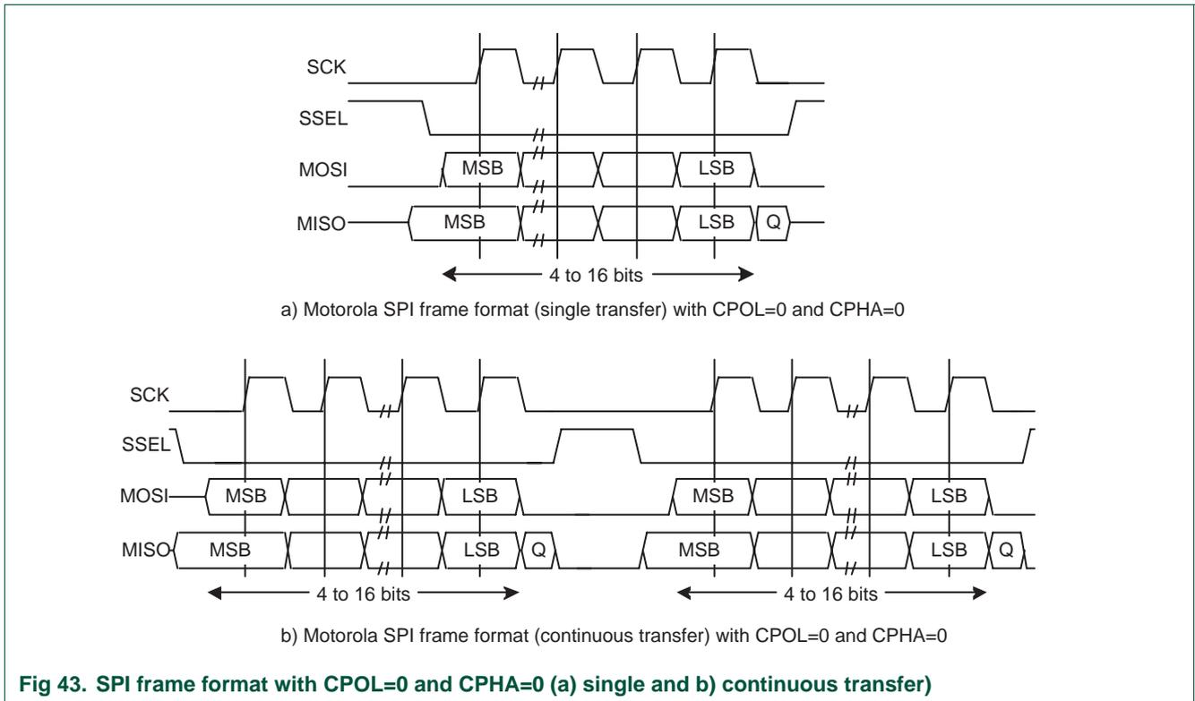
**Fig 43. SPI frame format with CPOL=0 and CPHA=0 (a) single and b) continuous transfer)**
