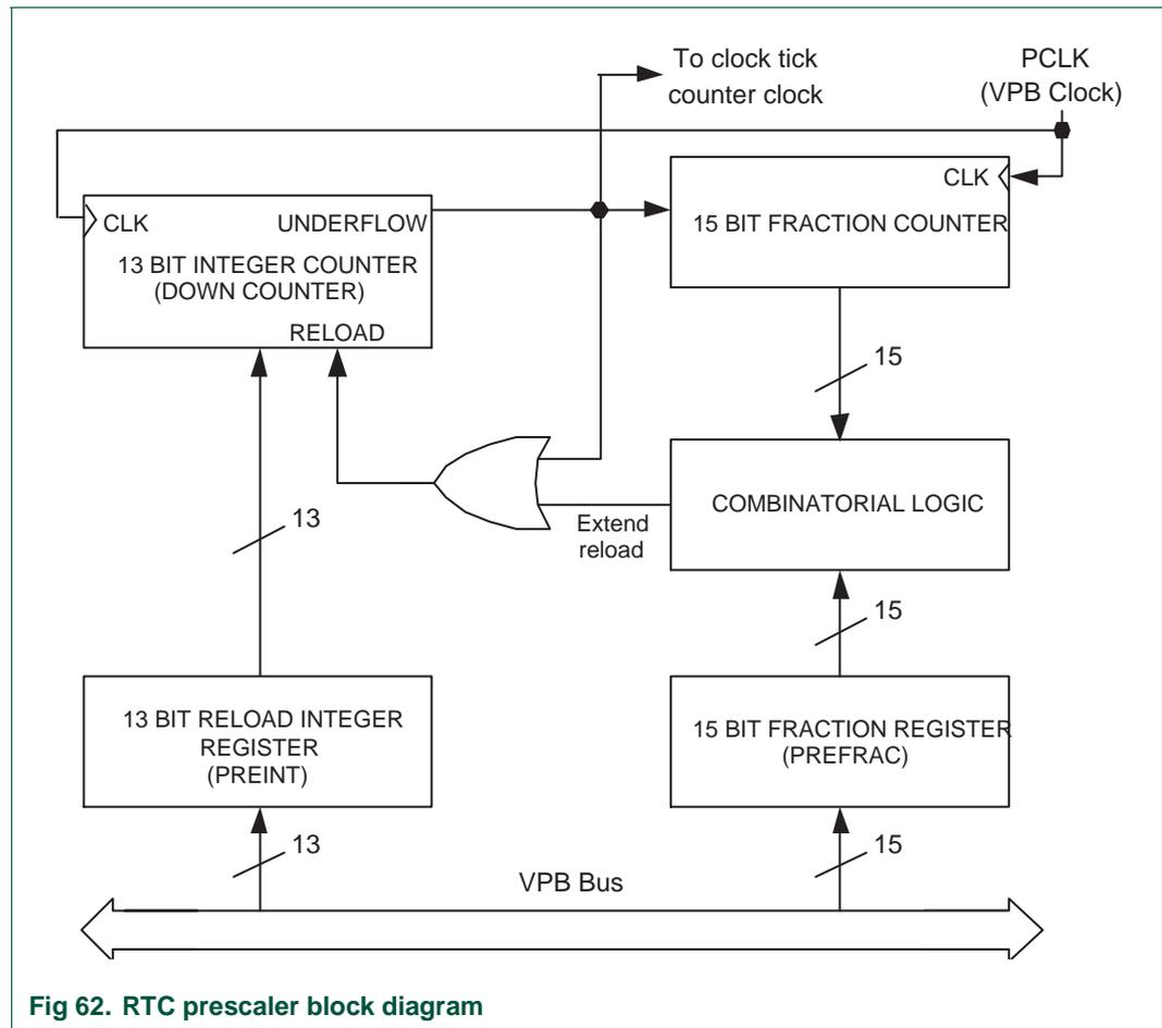
Fig 62. RTC prescaler block diagram
