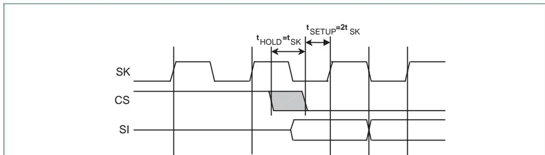
Fig 49. Microwire frame format (continuous transfers) - details
