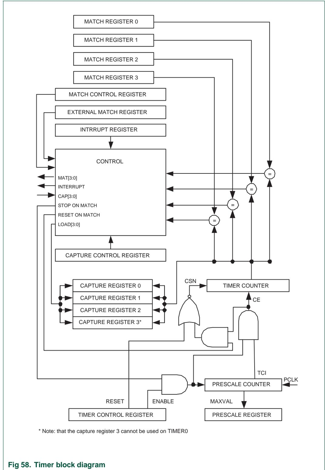
Fig 58. Timer block diagram
