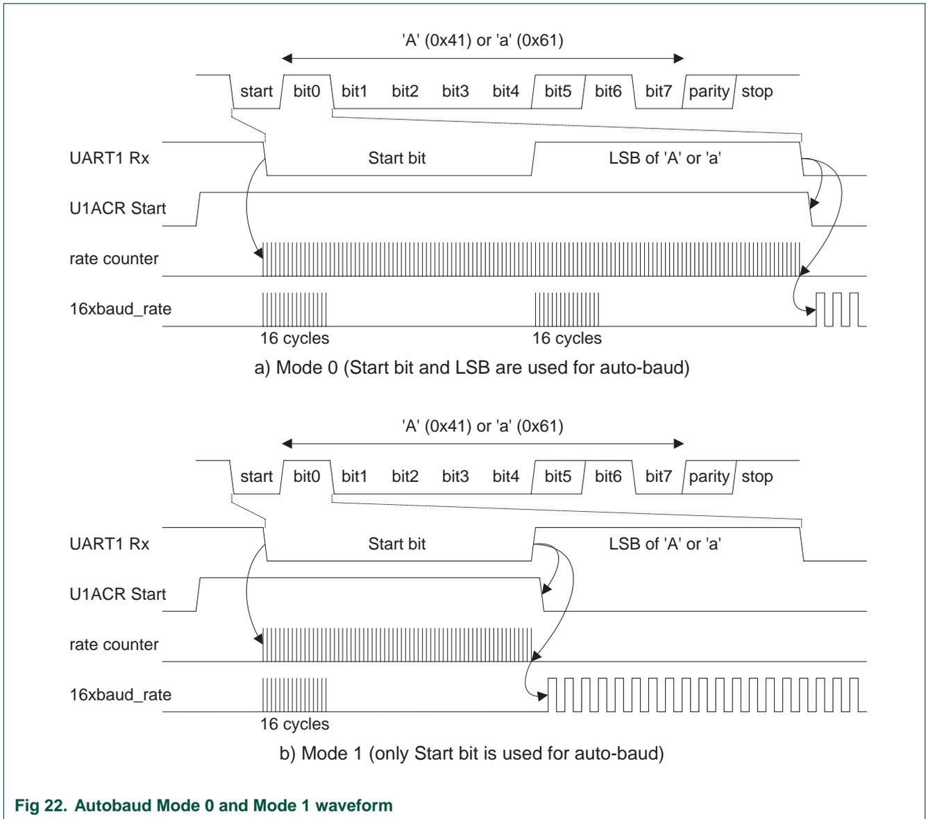
Fig 22. Autobaud Mode 0 and Mode 1 waveform
