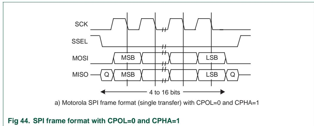
**Fig 44. SPI frame format with CPOL=0 and CPHA=1**
