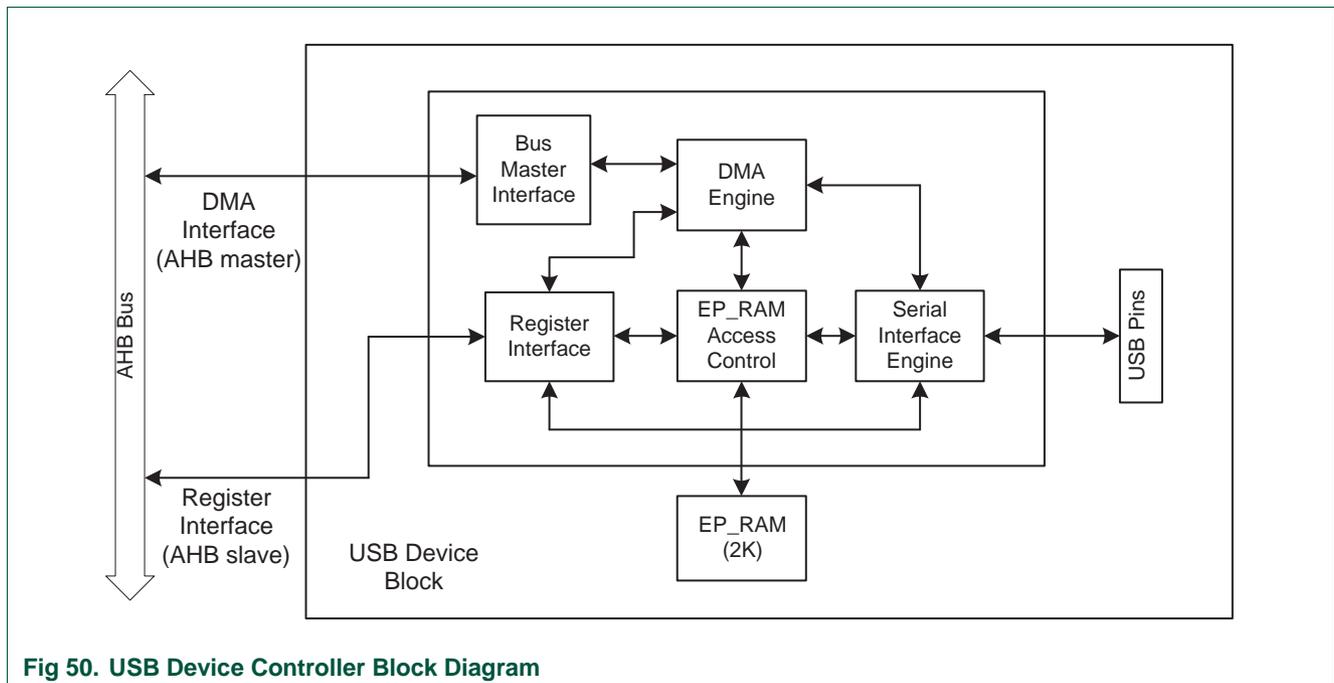
Fig 50. USB Device Controller Block Diagram
