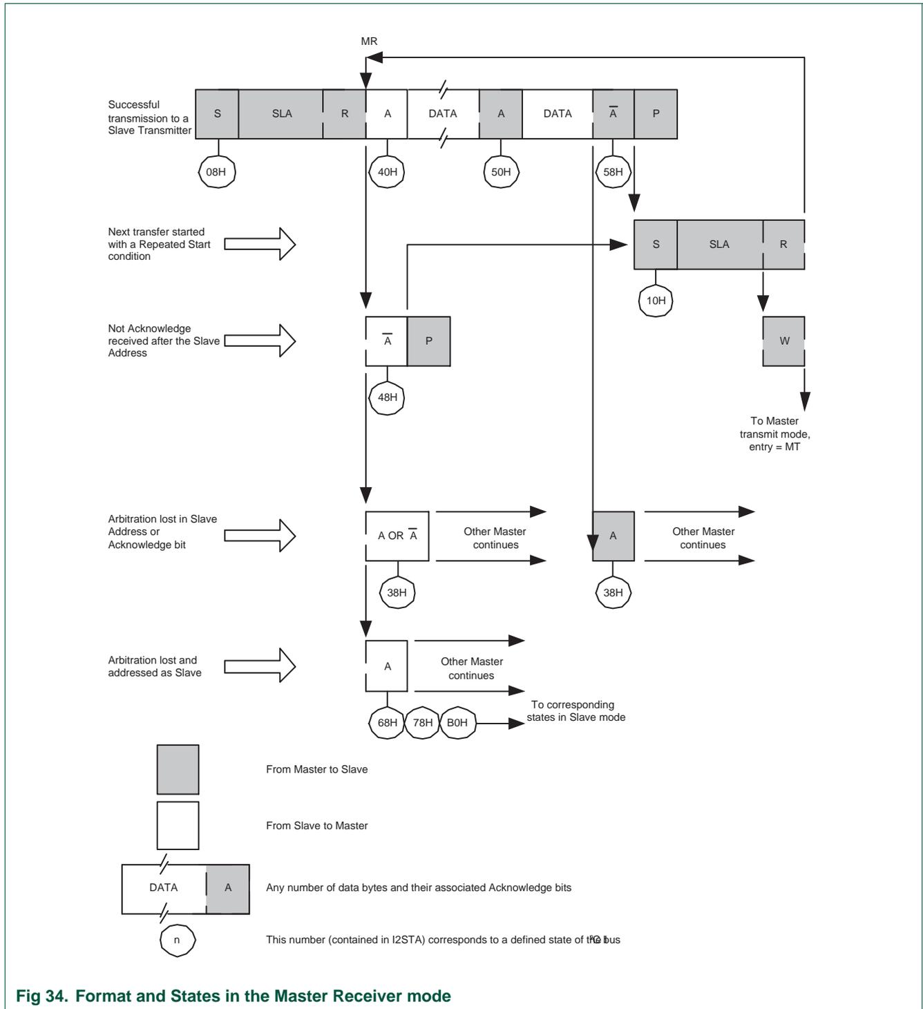
Fig 34. Format and States in the Master Receiver mode
