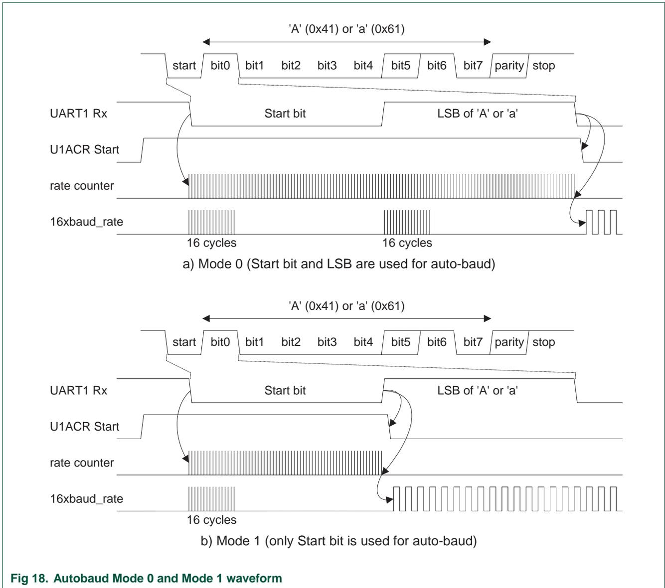
Fig 18. Autobaud Mode 0 and Mode 1 waveform
