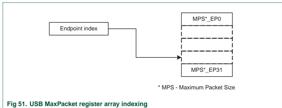
**Fig 51. USB MaxPacket register array indexing**
