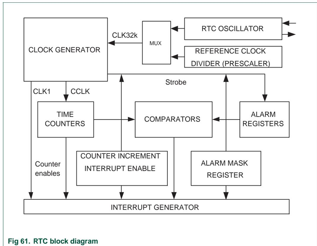
Fig 61. RTC block diagram
