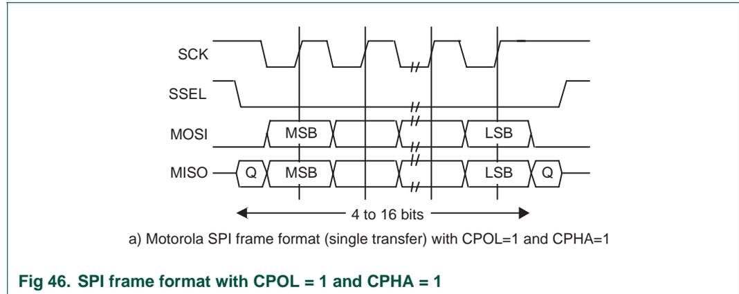
**Fig 46. SPI frame format with CPOL = 1 and CPHA = 1**
