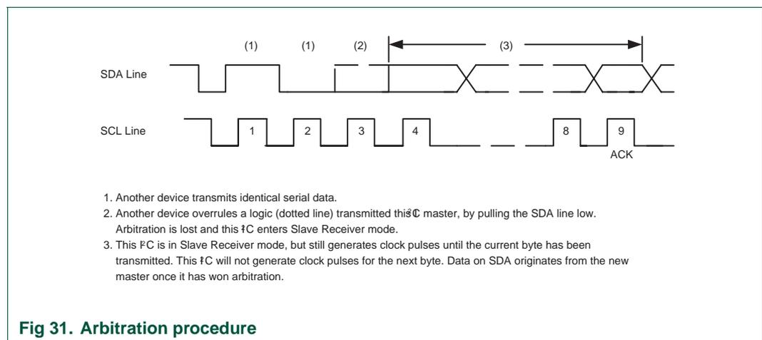
Fig 31. Arbitration procedure
