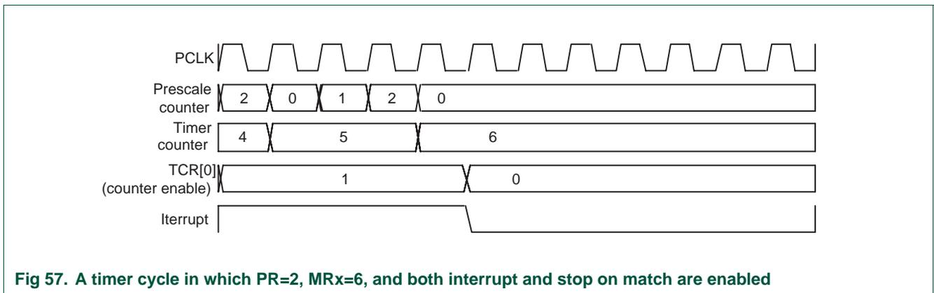
Fig 57. A timer cycle in which PR=2, MRx=6, and both interrupt and stop on match are enabled
