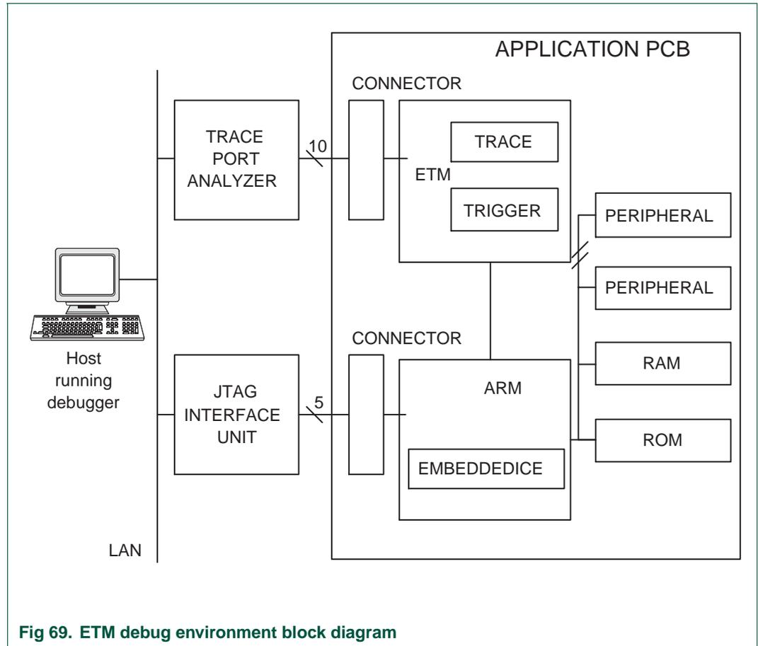
Fig 69. ETM debug environment block diagram
