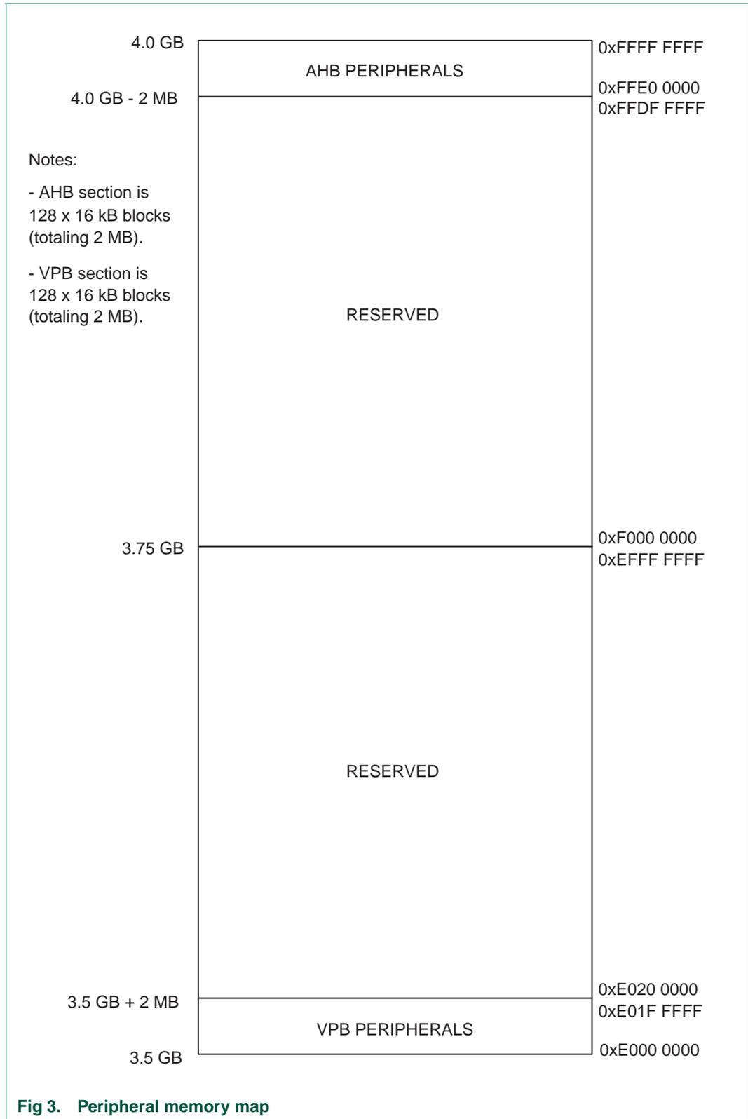
Figures 3 through 4 and Table 2 show different views of the peripheral address space. Both the AHB and VPB peripheral areas are 2 megabyte spaces which are divided up into 128 peripherals. Each peripheral space is 16 kilobytes in size. This allows simplifying the
