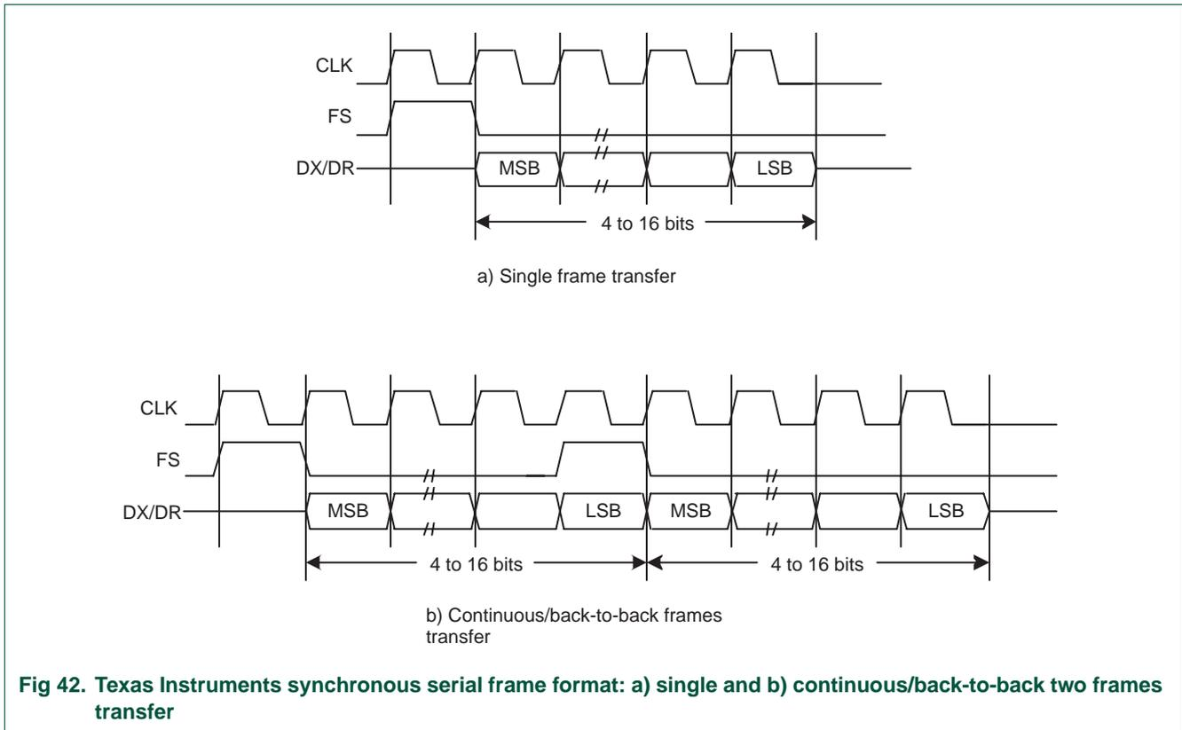
**Fig 42. Texas Instruments synchronous serial frame format: a) single and b) continuous/back-to-back two frames transfer**
