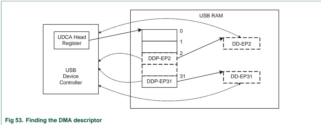
Fig 53. Finding the DMA descriptor
