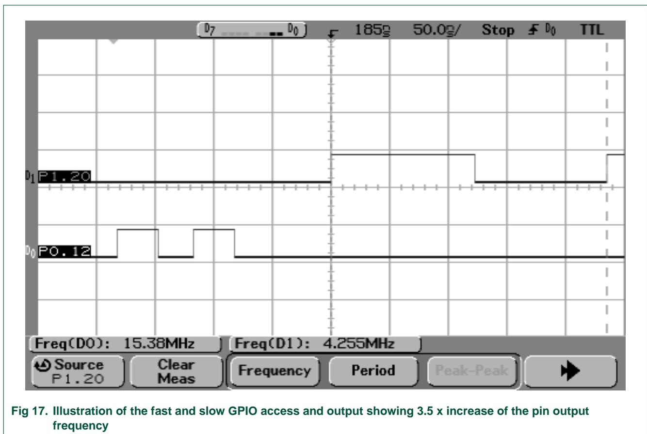
Fig 17. Illustration of the fast and slow GPIO access and output showing 3.5 x increase of the pin output frequency
