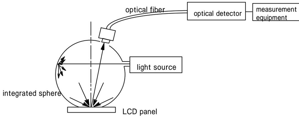
Fig.2 Measurement system-2
