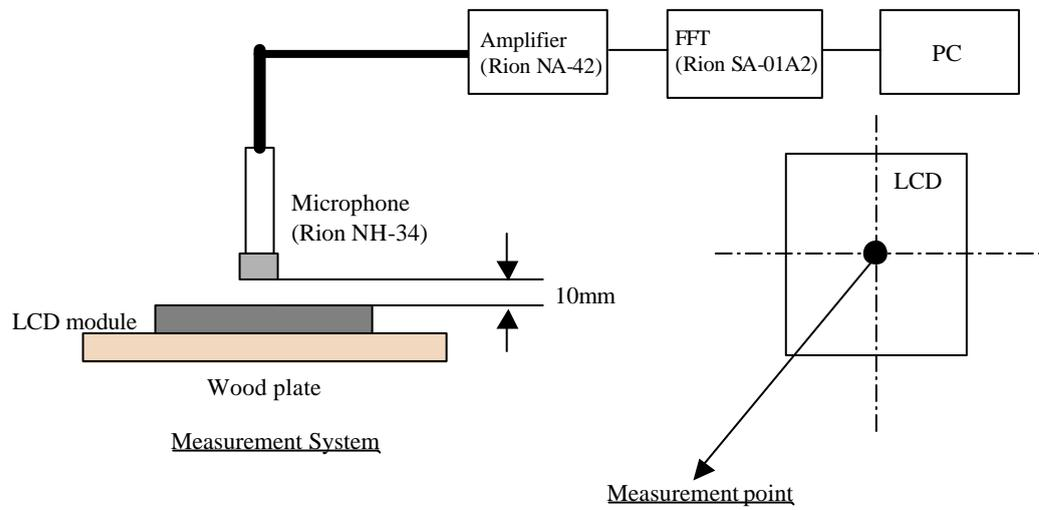
Fig.6 Measurement system-5
