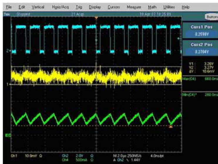
Figure 14. Ceramic 10µF 0603 (X5R) (Good)
