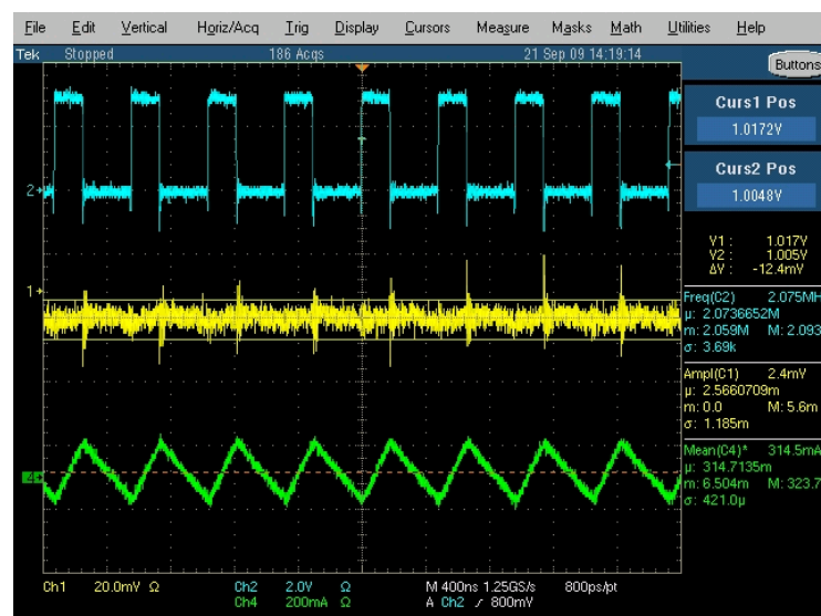
Figure 15. L=GLK2510P-2R2M, C=Ceramic 4.7µF 0805 X5R TDK (Ripple 12.4mV)
