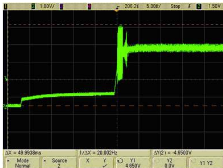
Figure 13. Input Voltage Overshoot >4V (Bad)
