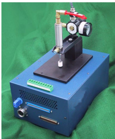
Figure 3-3: Theta JC Measurement Setup
