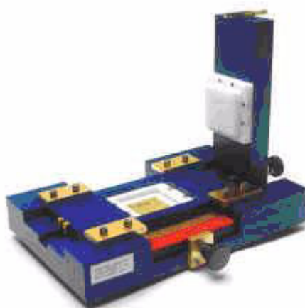
Figure 4-1: Altair BGA Fixture used for TDR measurement
