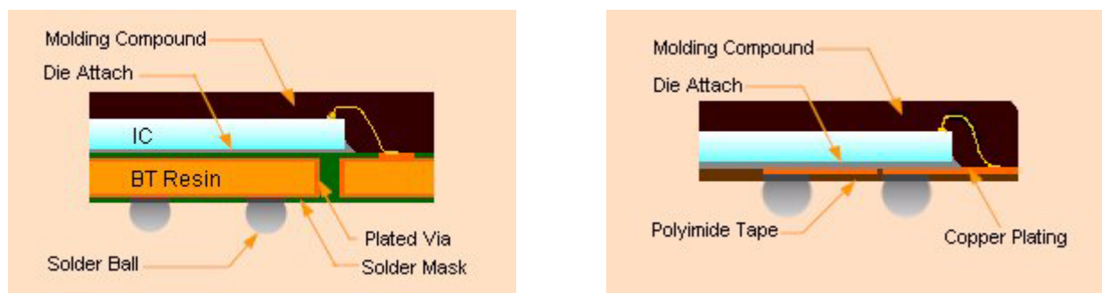
Figure 1-7: Rigid BT-based Substrate Chip Scale Packages, left; Flex-Based Tape Substrate, right
