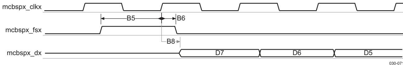
Figure 6-34. McBSP Rising Edge Transmit Timing in Slave Mode
